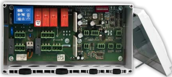
A plastic housing provides the external extensions, e.g. the HZS 541, with good protection.
